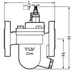
DIN type is shown. ASME type has welded on flanges.
